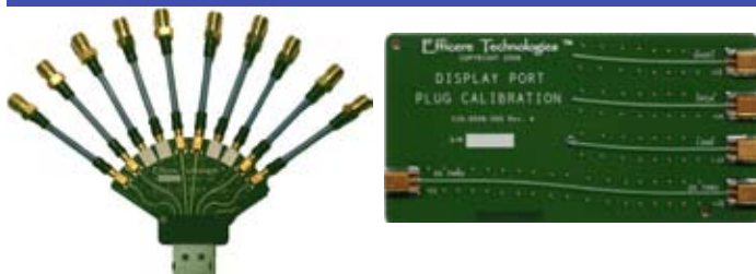
DisplayPort Plug and Plug Calibration boards. Plug board shown with 2" GPPO->SMA cables attached. (not to scale)
